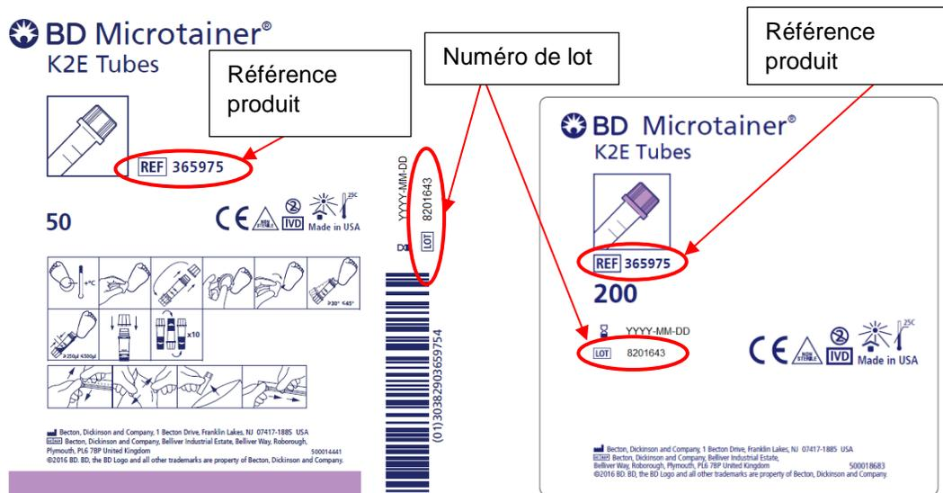
The diagram illustrates how to identify the product reference and lot number on two different labels for BD Microtainer K2E Tubes. Red circles and arrows highlight the 'REF 365975' and 'LOT 8201643' on both labels.
