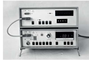
1977 DOSIMENTOR The first therapy dosimeter with field-effect transistors
