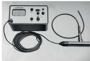
1955 SIMPLEX The first dosimeter with an electron tube
