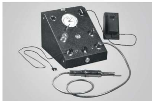
1922 Hammer Dosemeter The first X-ray therapy dosimeter based on an electrostatic relay
