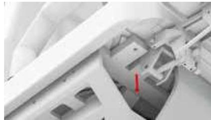
2. Unclip the hooks or elastics (depending on the model) at the back of the seat
