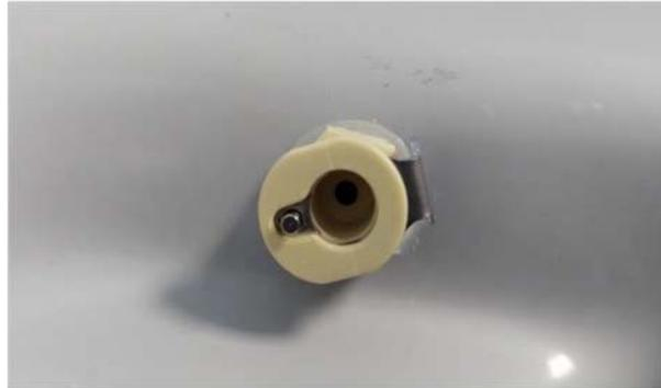
*Figure 1: Leak test socket***☒ Simulator tube cleaning:**
