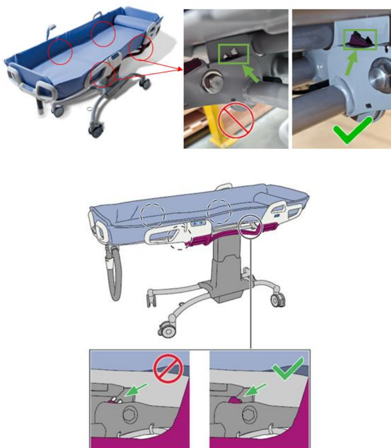
Figure 2 - Loquets "verrouillage incorrecte" et "verrouillage correcte"
